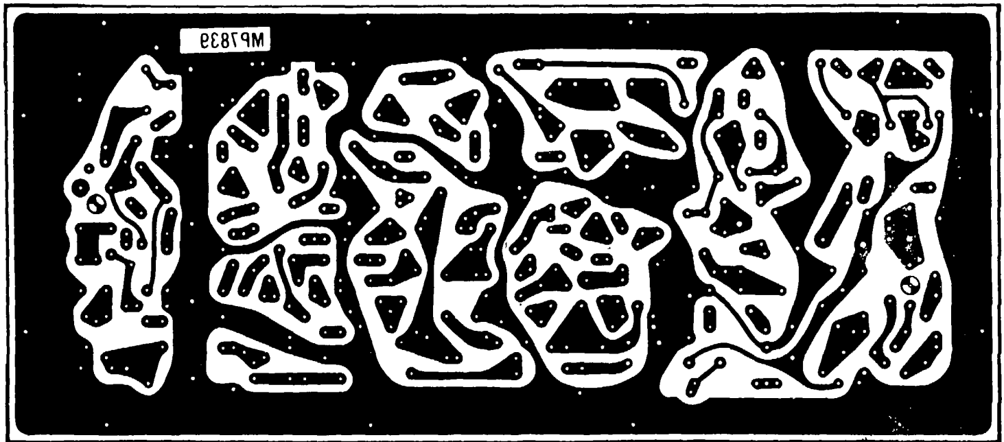
B WIRING ON BACK OF BOARD A3 (VIEWED THROUGH FRONT)
